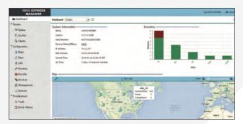
The system-level dashboard presents a map view of all the sites with inventory details for immediate visualization of the entire network. The site-level dashboard allows you to see the status of your access points and their radios, the client devices — including device type — connected to your access points, how much capacity is available, and more. And a drop-down box allows you to view information for your preferred timeframe — the last 30 minutes, the past two hours, or the last 24 hours.
