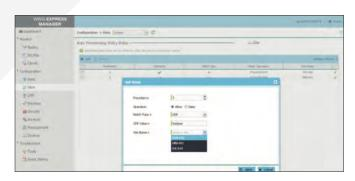
WiNG Express Manager's auto-provisioning feature allows you to deploy a multi-site WLAN network without any pre-staging. Policies can be defined for each site to match against parameters such as CDP/LLDP string, AP MAC, and IP address to place APs in a specific site and apply the appropriate configuration. As a result, the time required to deploy your WLAN infrastructure is significantly reduced.
