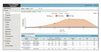
This ongoing system- and site-level log tracks and maintains a complete history of events that have occurred on your WLAN, providing valuable trending information as well as details you need to address a specific incident and prevent a reoccurrence in the future. You can inspect aggregated analytics at the system level or drill down to site-specific details for more granularity.
